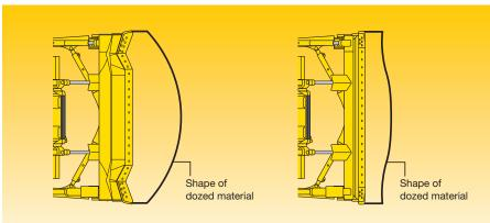
Up to 15% higher production with the improved Sigmadozer® blade (left), compared to conventional Semi-U blade (right)
