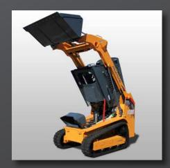
**SERVICEABILITY** All-new cab support lock eliminates the need for a second person when raising the ROPS/FOPS structure for maintenance.
