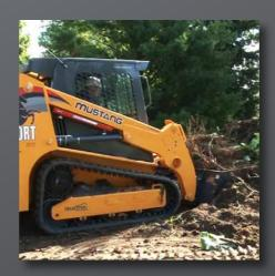
HORSEPOWER MANAGEMENT SYSTEM a monitors and adjusts the hydrostatic drive pump, resulting in tractive effort of 5371 kg on the 1750RT NXT2 and 5606 kg on the 2100RT NXT2.
